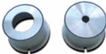
Figure 2. Cups for small spot analysis with 30 mm and 10 mm apertures.
